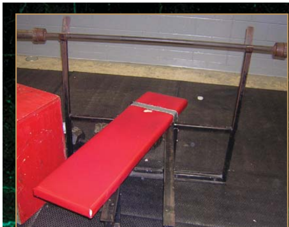
One of the most common reasons for lawsuits against weight rooms is inadequate equipment maintenance, as illustrated by this photo of a bench press taken recently at a high school weight room.
